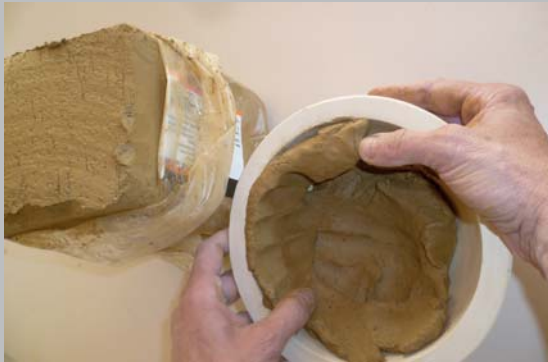
Forming an object from the body, e.g. a ball from a hemisphere plaster mould.
