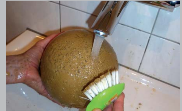
The leather hard body is finished under running water with a brush...
